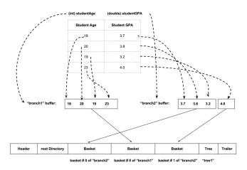
Fig. 6: Physical structure of the ROOT file storing the simple Table V
