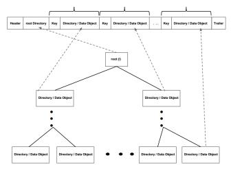
Fig. 2: Physical structure (top) and logical structure (bottom) of a ROOT file
