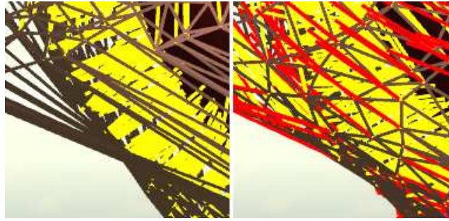
Figure 7: This figure illustrates the concepts of anchors, virtual anchors, and elastic relaxations where the skin is anchored on two neighboring segments. Skin vertices are connected by brown edges to form a triangle mesh. In the left image, skin vertices coincide with their virtual anchors, as no elastic relaxation has been done. In the right image, after elastic relaxation, the virtual anchor positions are unchanged, while the skin vertices have been redistributed more uniformly. In both images yellow lines connect skin vertices to their muscle anchors. In the right image red lines connect the skin vertices to their virtual anchors, showing the displacement necessary to equalize spring forces.
