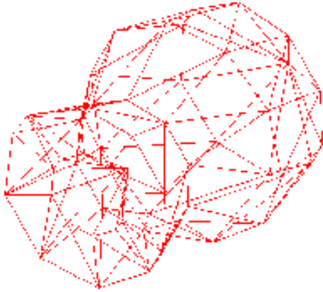
Figure 5: Triangulated scattered data points
