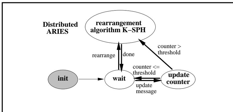
Figure 7: The finite state machine in member nodes corresponding to a distributed implementation of ARIES.
