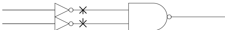
Figure 2.2: Example of a nonpropagatable non-feedback short, when the short causes wired-AND behavior.
