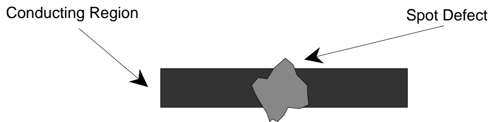
Figure 2.5: Example of a defect causing a break fault.
