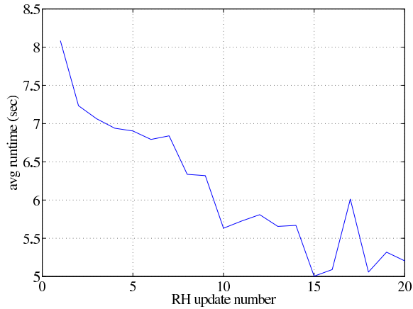
Figure 7: Average run time versus receding horizon update number, for the three distributed optimal control problems solved in parallel.
