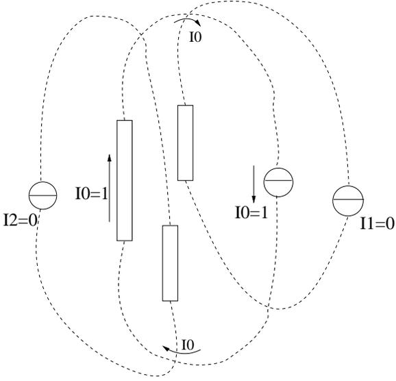
Fig. 1. Partial inductance extraction under PEEC model (The dashed line means the current return loop and the current sources are at infinity.)
