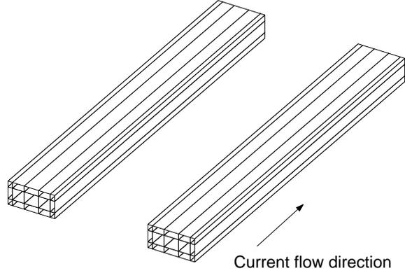
Fig. 3. An example of non-uniformly mesh 2 conductor segments into  $2 \times 5 \times 3$  filaments
