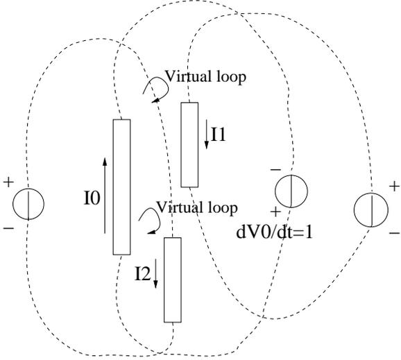
Fig. 2. Partial reluctance extraction by its physical meaning (The dashed line means the current return loop and the voltage sources are at infinity.)
