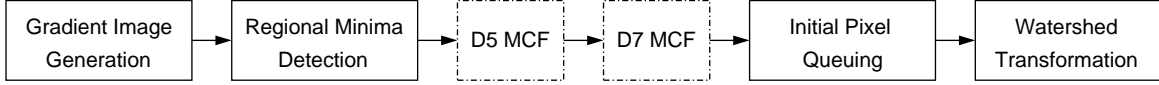
Figure 4: Modified process flow of the immersion simulation-based WST. This figure shows the stages where D5 and D7 MCFs are applied.
